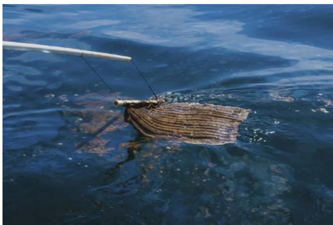
Oleo Sponge pads were secured to long PVC pipe for deployment on the oil sheen and easy recovery (see photos). Numerous runs were performed, using both very fresh and somewhat weathered oil. In all cases, Oleo Sponge successfully lifted the sheen from the water, leaving behind no visible oil. Videos of this process, submitted to accompany this report, provide compelling evidence for the efficacy of this technology for oil sheen mitigation.
